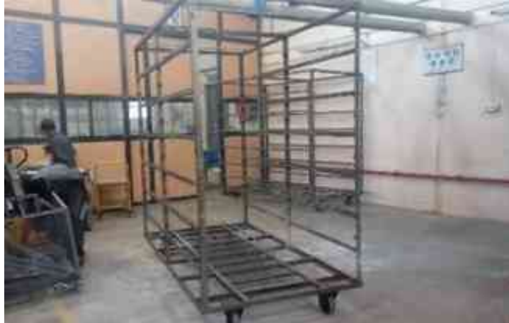
High LPG & Electricity consuming 'MS' trolleys
