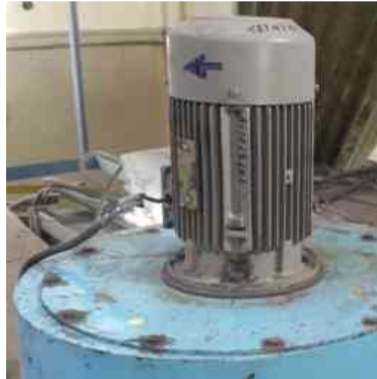
Electric Motor with IE3 class
