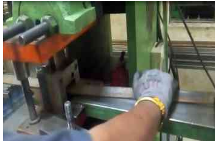
Die designed to cut in single stroke)
