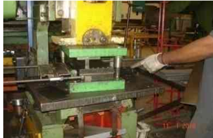
Press tool for strip(W-300) parting
