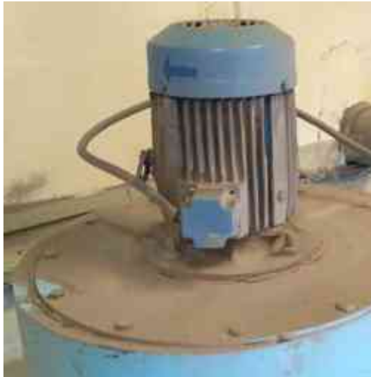
Electric Motor with IE1 class
